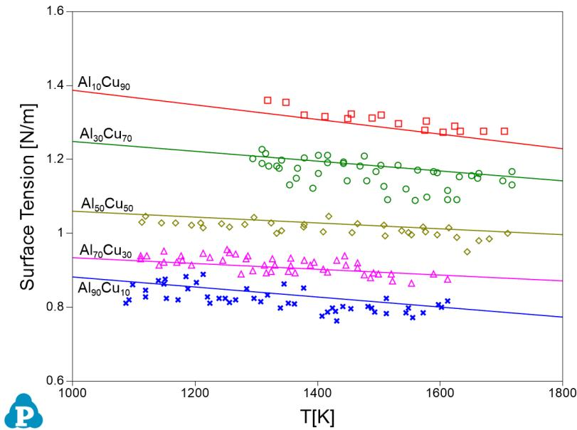
**Figure 3.3:** Surface tension of Al-Cu alloys
