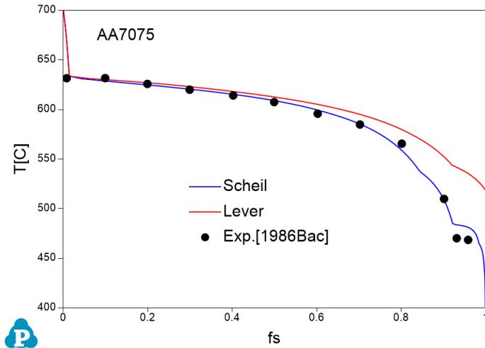
**Figure 1.10:** Comparison between calculated and experimentally measured solidification paths of AA7075 aluminum alloy
