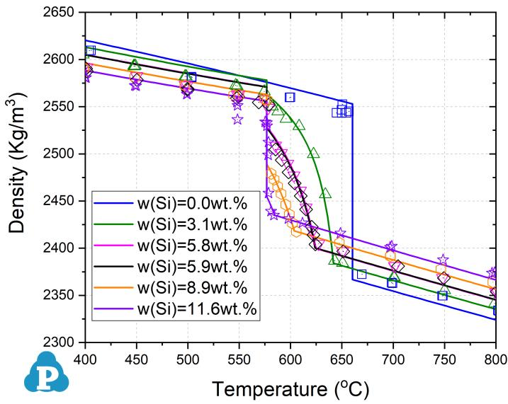
**Figure 3.2:** Density of Al-Si binary alloys [2001Mag]
