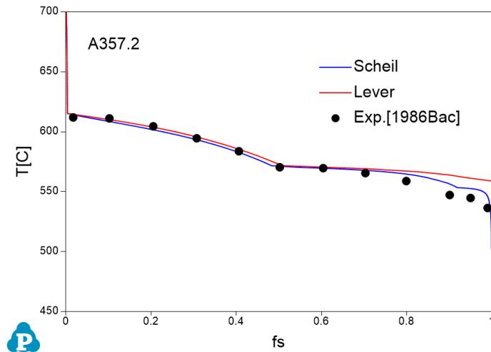
**Figure 1.8:** Comparison between calculated and experimentally measured solidification paths of A357.2 aluminum alloy
