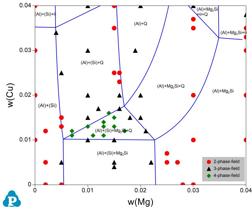
**Figure 1.1:** Comparison of a calculated isothermal section of Al-Cu-Mg-Si at 1.8wt%Si and at T=500 °C with the experimental data [1962Smi]
