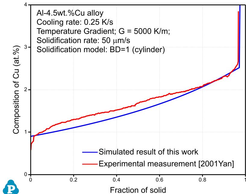
**Figure 2.7:** Comparison of simulated and experimentally determined Cu composition profile within the Fcc matrix for the Al-4.5wt.%Cu alloy at the cooling rate of 0.25K/s
