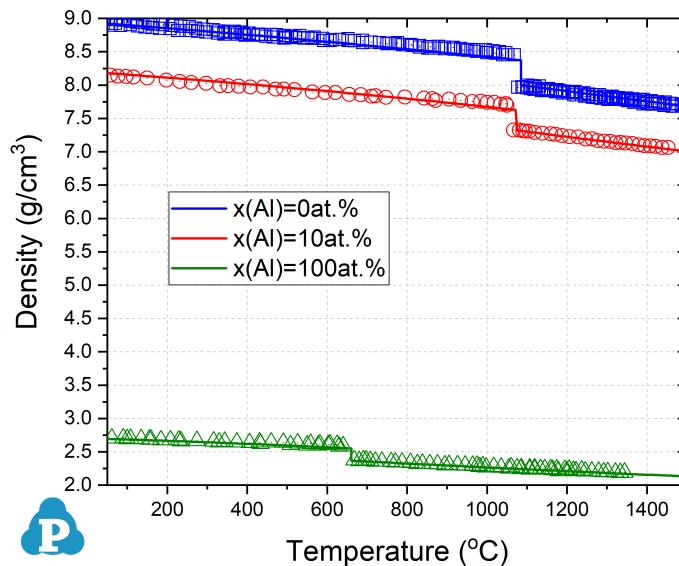
**Figure 3.1:** Density of Al-Cu binary alloys [2013Kur]
