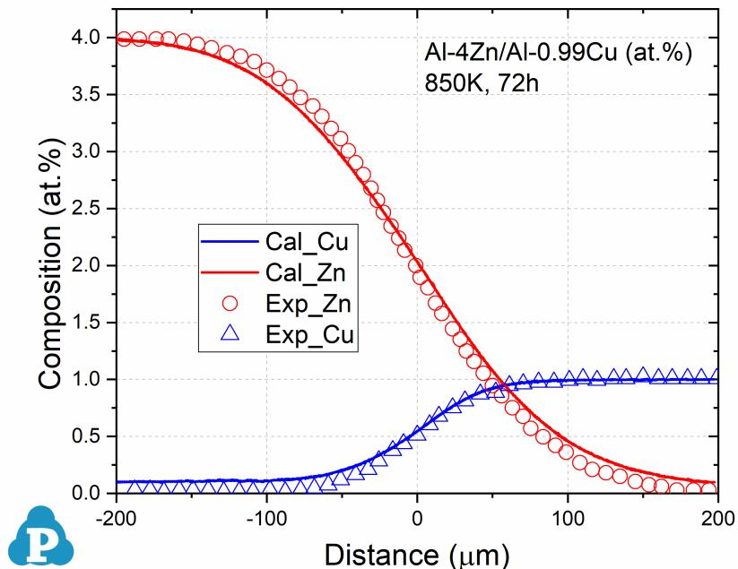
**Figure 2.2:** Concentration profile of Al-4Zn/Al-0.99Cu (at.%) annealed at 850K for 72h
