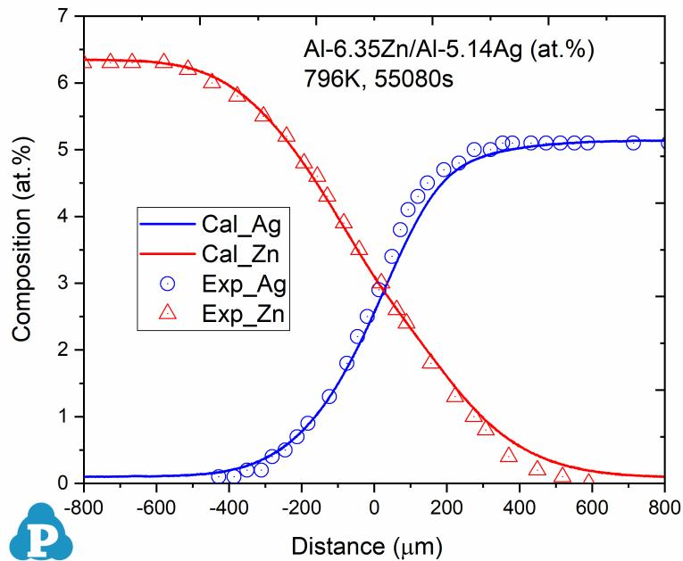
**Figure 2.1:** Concentration profiles of Al-6.35Zn/Al-5.14Ag (at.%) aged at 796K for 55080s
