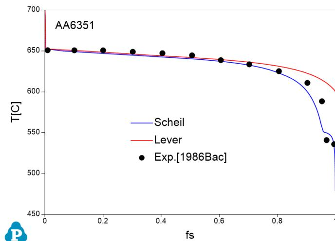
**Figure 1.9:** Comparison between calculated and experimentally measured solidification paths of AA6351 aluminum alloy
