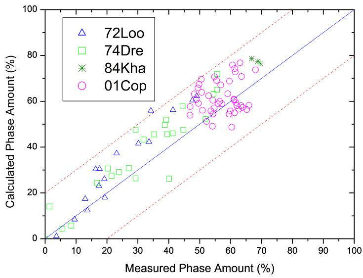
**Figure 1.3:** Comparison between the calculated and experimentally measured amounts of the  $\gamma'$  phase
